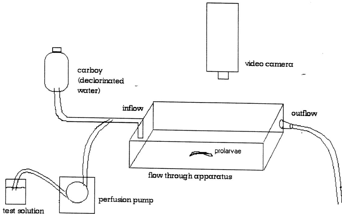
Fig. 2 Flow through apparatus and experimental setup.
