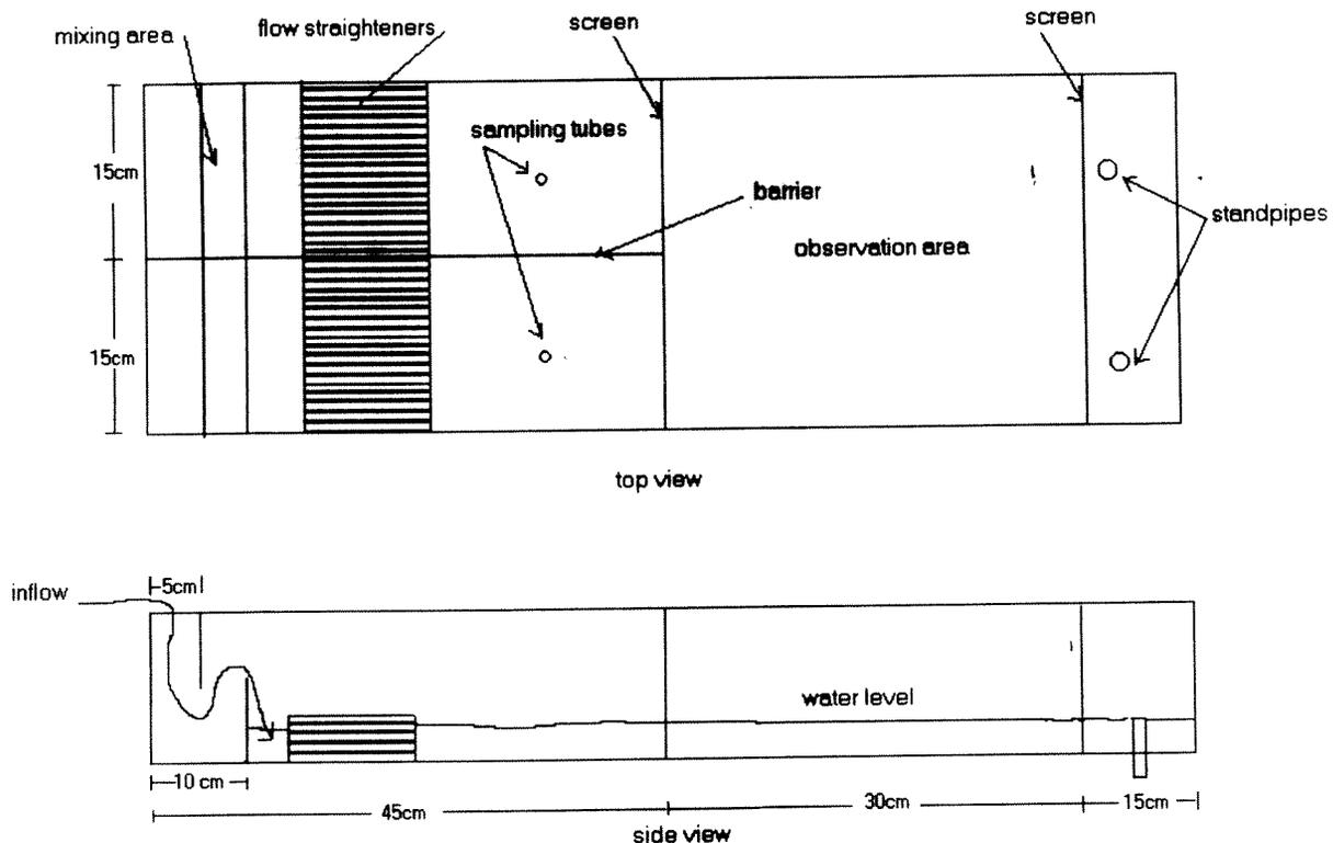
Fig. 6.1 Diagram of the ammocoete behavioral apparatus.
