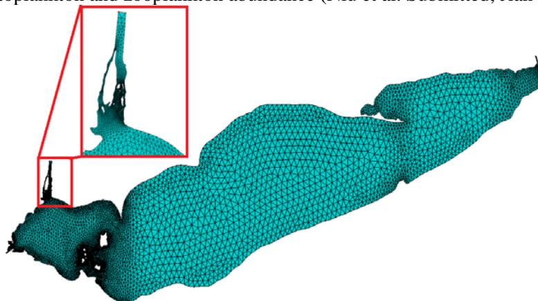
Fig. 2. Schematic of unstructured grid used to model Lake Erie hydrodynamics. Model resolution was 0.017 km to 7.77 km
