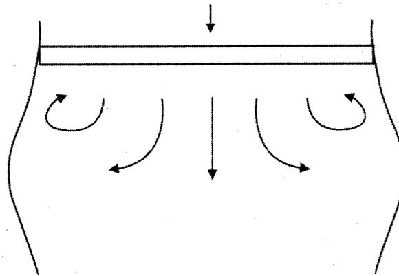
Figure 1. Schematic presentations of the hydraulic jump that can occur at the base of low-head barriers. a) Side view showing vertical vortices. b) Top view showing horizontal vortices. Based in part on Leutheusser and Birk (1991).
