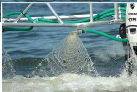
An innovative granular baylucide sprayer boat employs a high pressure spray system and GPS to effectively target lentic areas on the St. Marys River system.
