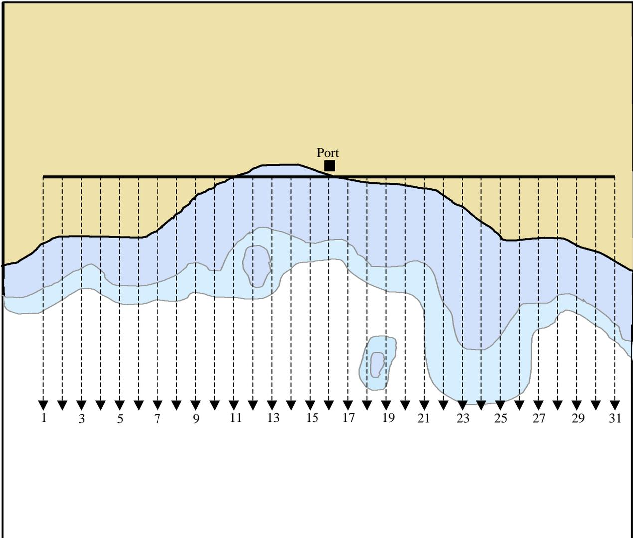
Figure 3. Generalized illustration of 31 possible sampling vectors originating from a base line drawn through a stylized port location. The thick black line runs roughly parallel to the shoreline with the port at its center. Vectors are 1.8 km apart and run perpendicular to the base line. Each year, sampling nets will be set within three depth ranges (15-30 m; 31-45 m; and 46-60 m) along two randomly selected vectors.
