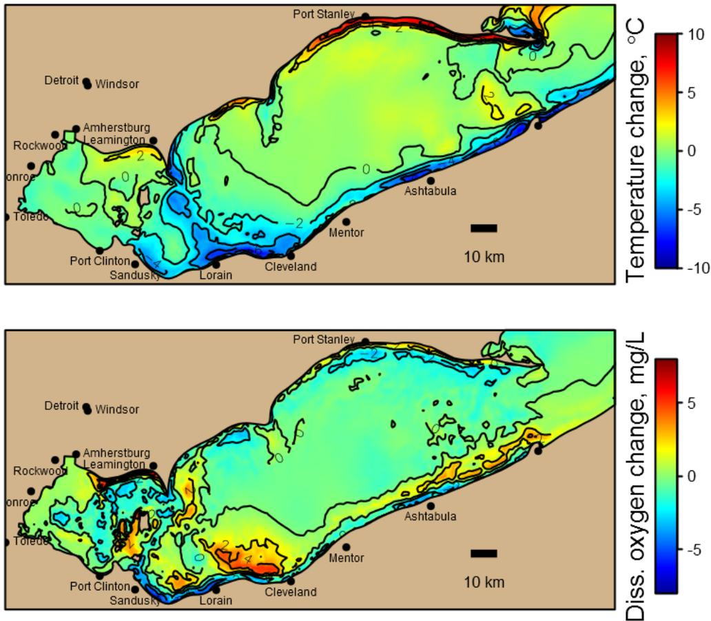
Figure 6. Image from the Lake Erie hypoxia change in bottom temperature and dissolved oxygen forecast animations as generated by the experimental hypoxia forecast model.
