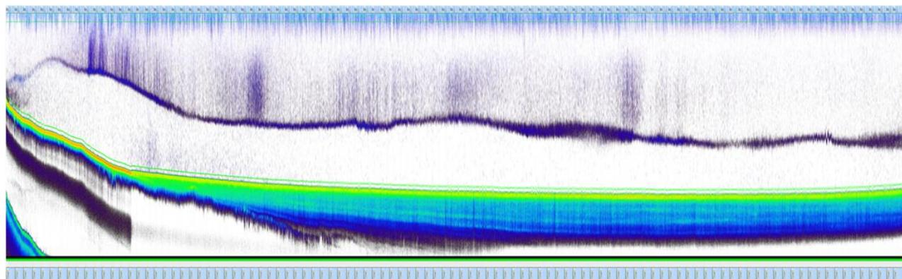
Figure 3.2.7. Echogram files generated from Echoview<sup>®</sup> software version 5.1 that show total back scattering ( $S_v$ ) along transects in the central basin, 2014.
