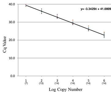
The mean PCR efficiency of the assay was 99.4 ± 0.06% (SD), with a 95% confidence limit of 0.0296 (R<sup>2</sup> = 0.994).
