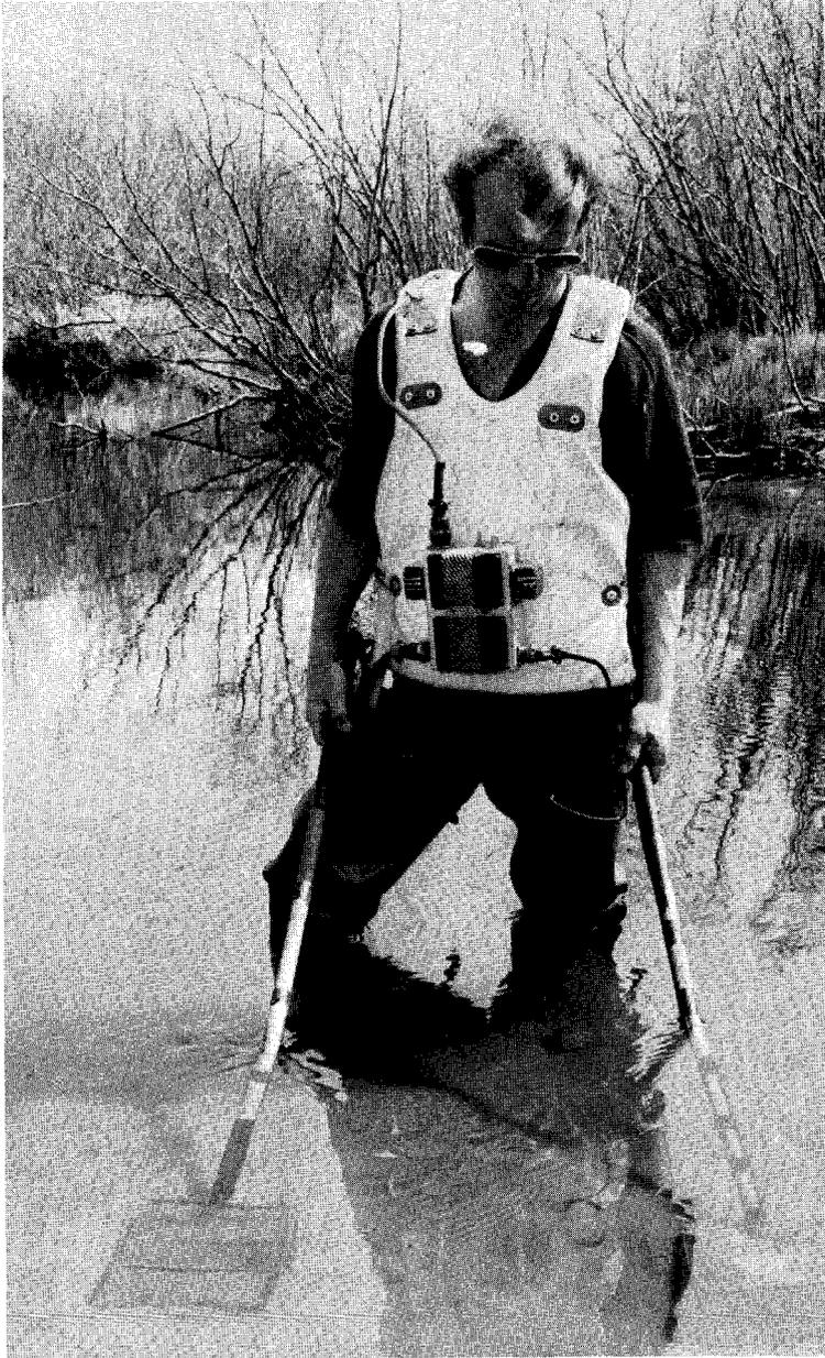
Fig. 9. Collecting ammocetes with a transistorized back-pack shocker.
