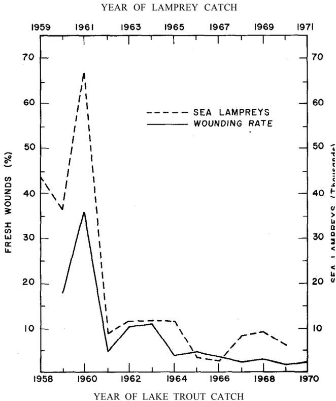
Fig. 17. Catch of spawning-run sea lampreys at 16 United States barriers, 1959-71 (scale at top), and the corresponding wounding rates for lake trout 610 to 632 mm (24- to 24.9-inches long), 1958-70 (scale at bottom). Wounding rates, from the fall of the year, are set forward 1 year to correspond with the catch of lampreys that caused the wounding.
