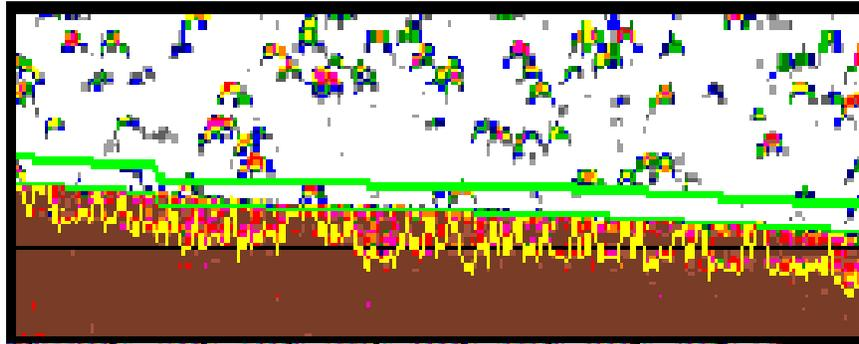
Transducer motion results in a change in the orientation of the transducer beam, relative to the insonified targets, between transmission and echo return. Targets insonified on-axis may be received off-axis or vice versa. Similarly, the return signal from targets insonified at the edge of the beam may be lost. The effect of transducer motion on data is complex, but includes:
