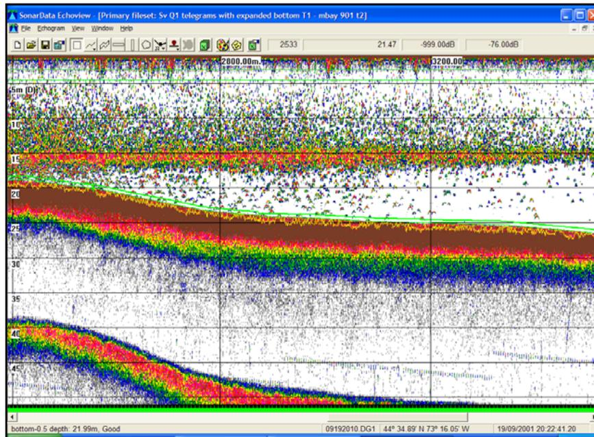
Fig. 11b. Expanded echogram showing high noise detected at the surface.
